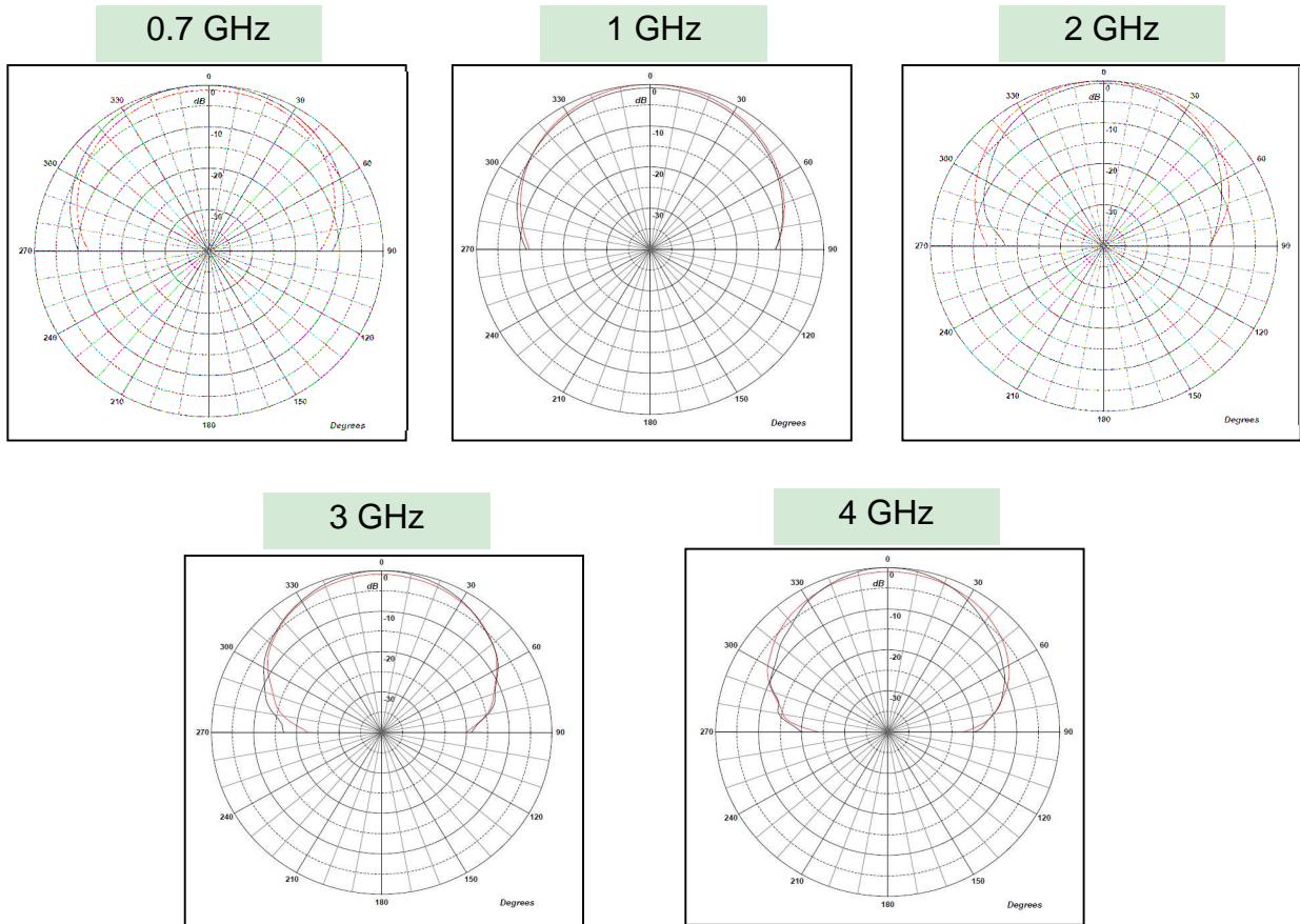
\* Patterns measured using a linear source antenna , Polarisation refers to the polarisation of the source horn. On patterns the **Red trace = Horizontal Pol source, Black trace = Vertical pol source**
