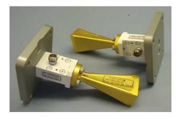
Note that the connector upper frequency suggested limit is 65 GHz
