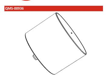
Typical Specification Frequency 2 to 40 GHz Connector K-Type Female **VSWR** < 2.0 :1 (Typically) Gain -7.7 to 4.4 dBi **Axial Ratio** 0.1 to 4.9 dB 3 dB Beamwidth 57.4 to 131.5 degrees 10 dB Beamwidth 110 to 224 degrees 2W CW Power Size & Weight 51mm Diameter, 44.4mm Length.140g nominal Mounting 3 x M3 holes (rear mounted) on a Ø38.1 PCD **Environmental** MIL-STD-810H
